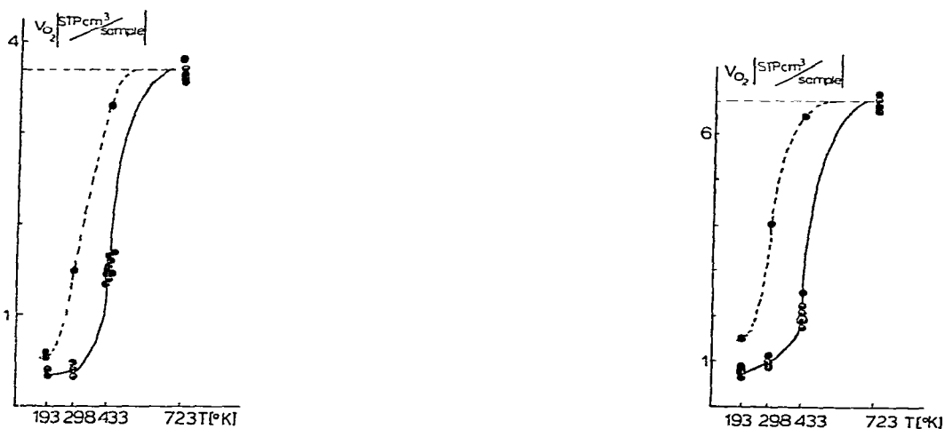
Fig. 1. Oxygen sorption on a reduced 1% iron catalyst as a function of temperature (continuous curve). Oxygen sorption after prolonged contact with oxygen for various temperatures (dashed curve). The points for the dashed line were obtained in an indirect way, based on additional oxygen sorption at 723°K after prolonged contact of a sample with oxygen at various temperatures. The amount of oxygen sorbed during this contact (dashed line) was determined as the difference between oxygen sorption at 723°K (no earlier contact of a sample with oxygen) and additional oxygen sorption at that temperature (after contact with oxygen at the investigated temperatures). The horizontal dashed line corresponds to the value of oxygen sorption at 723°K, which was assumed for estimating individual points on the dashed curve.
